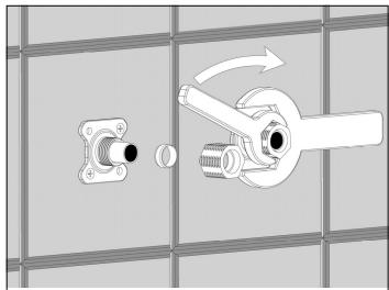
Slide the compression olive over the pipe and fit the hexagonal collar by tightening with a spanner. It is important that the brass bracket is supported by another spanner while tightening takes place.
