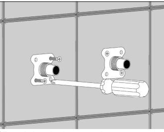
Offer up the brass brackets, ensure they are square and level, mark and then drill holes in the tiles or wall surface with a suitable drill. Insert wall plugs to suit the screws you have chosen (not supplied). Fix the brackets in place with at least two screws in each (preferably four in each).
