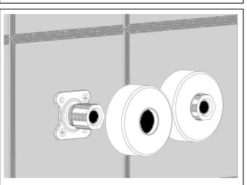
Spin the chrome plated covers on to the hexagonal collar and the connections are ready for the installation of the bar shower mixer.
